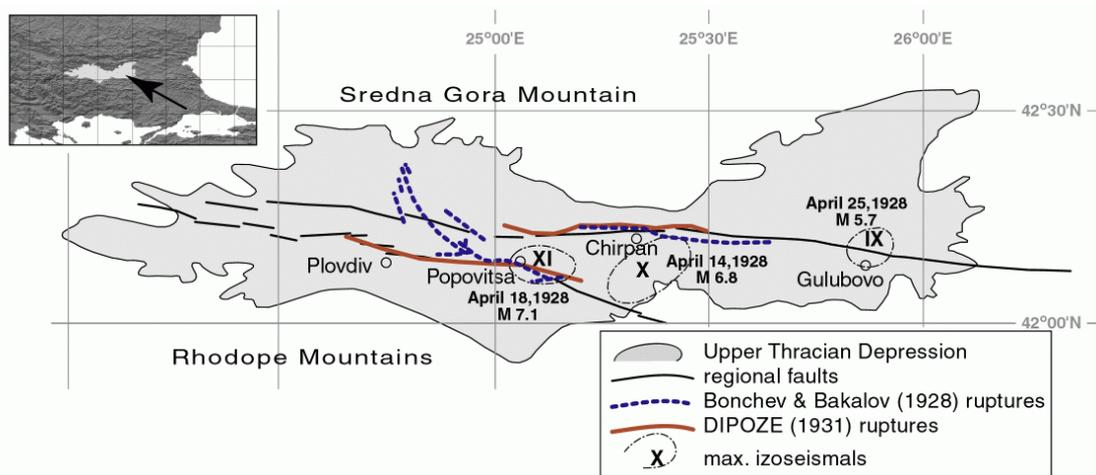
Figure 1. Map of the 1928 surface ruptures in the Upper Thracian Depression.
