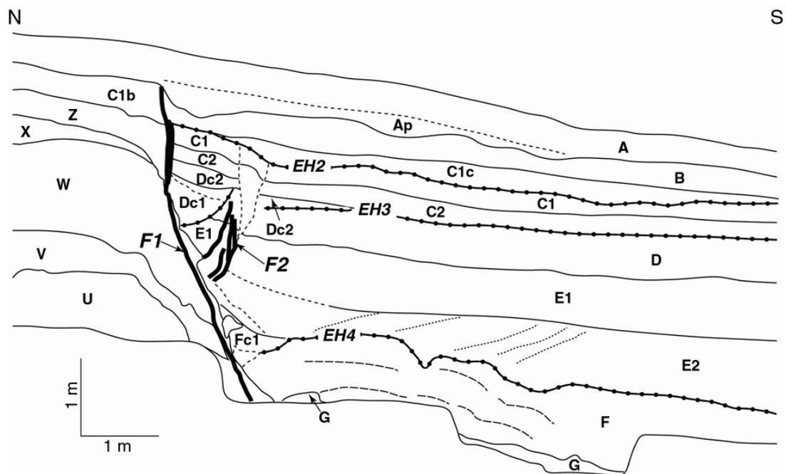
**Figure 3. Fault zone on east wall of Cherna Gora trench.**
