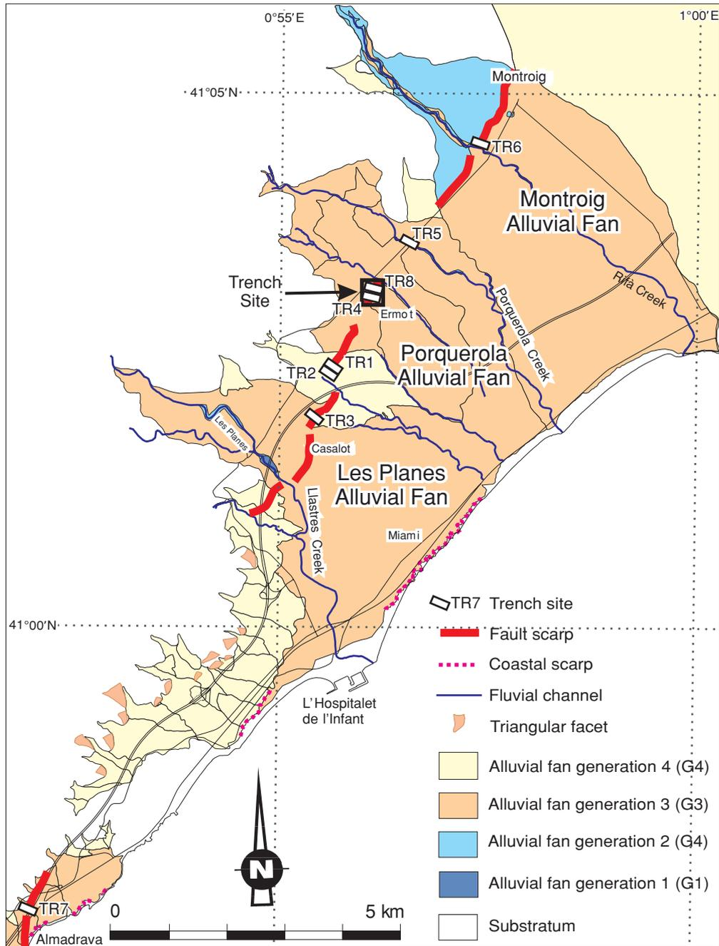
**Fig. 2.** The El Camp basin geomorphological map (modified from Masana *et al.*, 2001b). Location is shown in fig. 1. The map shows the distribution of the different alluvial fan generations as well as the zones where the fault scarp intersects the different alluvial fans.
