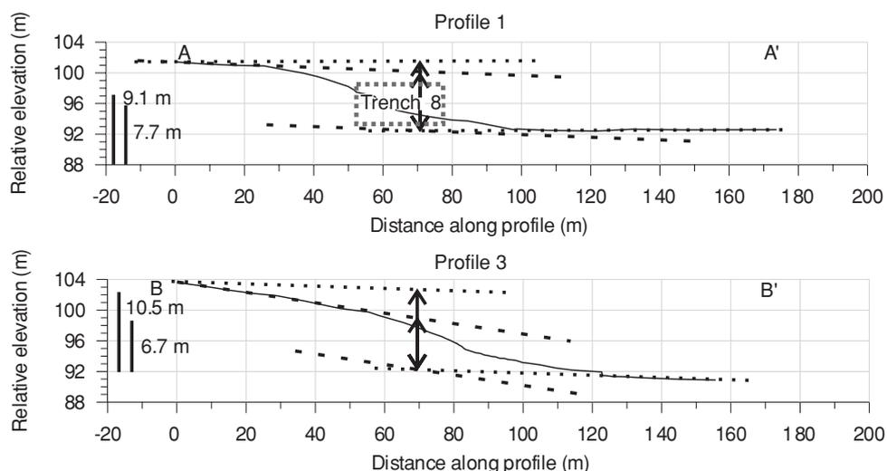
**Fig. 4.** Topographic profiles 1 and 3. A maximum and a minimum offset are plotted for each profile, taking into account that the original fan slope surface could correspond to the surface on the downthrown (dotted line) or upthrown block (dashed line). The position of trench 8 is projected on profile 1. The location of the two profiles is shown in fig. 3. The vertical scale is exaggerated.
