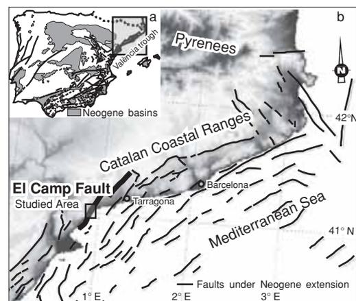
**Fig. 1.** Location maps: a) location of the Catalan Coastal Ranges within the Iberian Peninsula. The map shows the Neogene basins and the faults with Neogene extension; b) Location of the El Camp Fault within the Catalan Coastal Ranges. The map shows the *en échelon* array of NW-SE Neogene listric faults in the Catalan Coastal Ranges.
