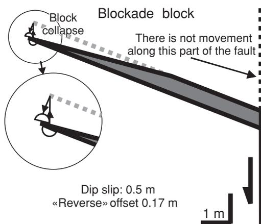
**Fig. 8.** This figure shows how a tensional fracture with an associated hollow and a post-collapse reverse geometry on a strongly vertical normal fault is produced (explained in the text). Semicircles identify homologue points and arrows indicate the movement of the block.
