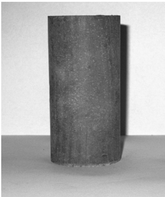
Fig. 2. Test specimens of the plastic ternary mixture after 28 days of curing
